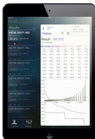
Typical CFPP result of a -37°C test.
