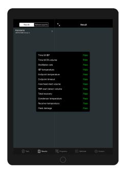
"Pass / Fail" test validation helps operators process only those results that are obtained from correctly executed tests. The validation is based on pre-defined method limits such as "Time to IBP", "IBP/FBP temperature", "Condenser/receiver temperature", distillation rate, etc.
