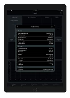
Create and customize program settings for specific products, or simply "Optimize" the program based on automatic suggestions from the previous test. Easy 1-step program creation based on pre-defined method settings. Requires authorized user and password.
